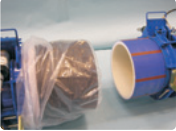
The coupler is placed on the end of the pipe
