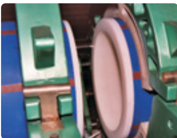
ProFuse is butt fused using standard equipment
