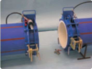
The pipe ends are rounded, if appropriate
